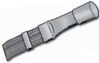
All metal tool straightens and cleans condenser and evaporator fins. Works on all units. Heavy-duty spring wire bristles automatically adjust to all spacings. Tension adjustment band allows maximum rigidity and ease of operation. Straightens even the most severely damaged fins.
